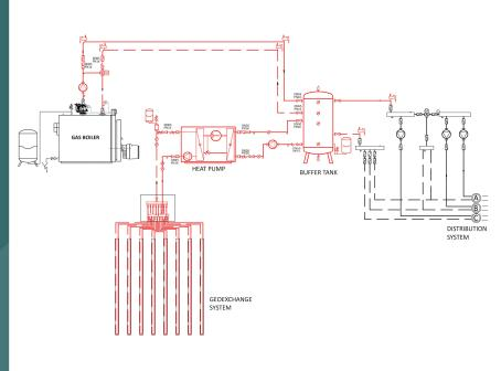
Choosing the right bivalent air temperature point and type of hybrid system is most suitable for retrofit projects in older buildings where a distribution system (radiators or fancoils) and gas boiler is kept (black lines on Figure) and a hybrid system with a heat pump is employed inside the existing engineering room (red lines on Figure).
