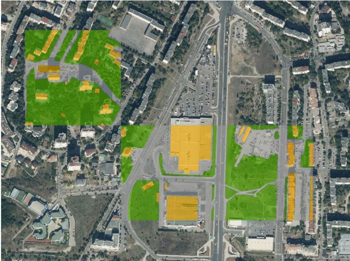
Figure 26: Example of classified land cover types in the spatial areas (Sealed surfaces - grey, buildings - yellow, vegetation - green). Source: Good Practices Report
