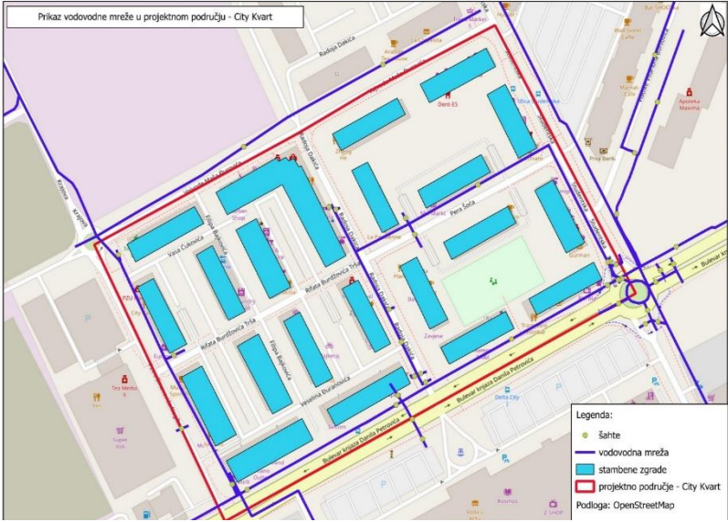
Figure 5: City Kwart water supply network
