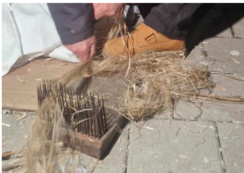
Figure 12: Traditional hackling of hemp fibers using a metal comb
