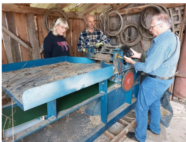
Figure 19: Conventional decorticator operated by the ZAKON Cooperative.
