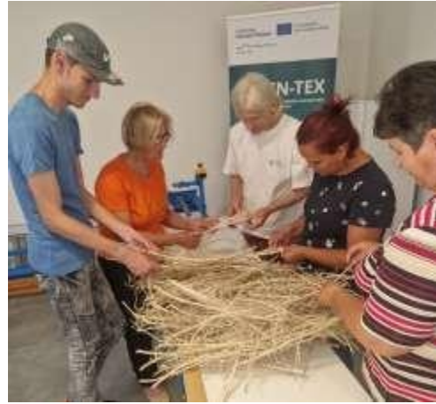
Figure 15: Drying of hemp stalks, followed with manual separation of hemp fibres from hurd
