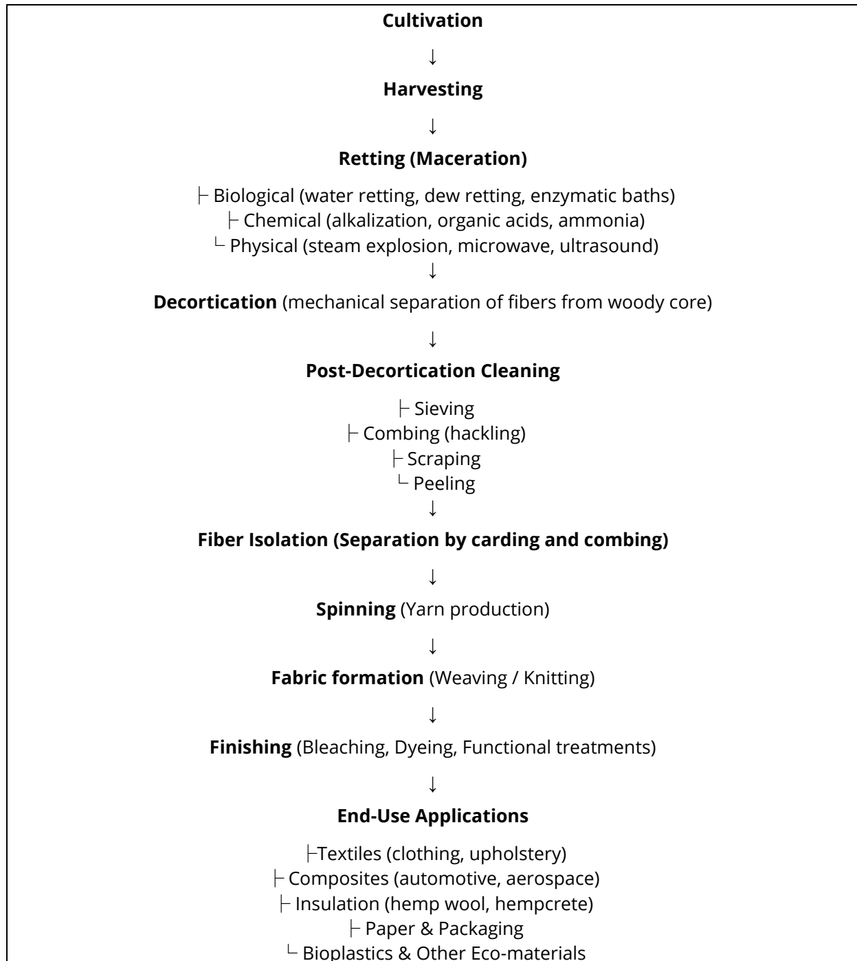
Figure 10: Hemp processing scheme, adapted from [35]
