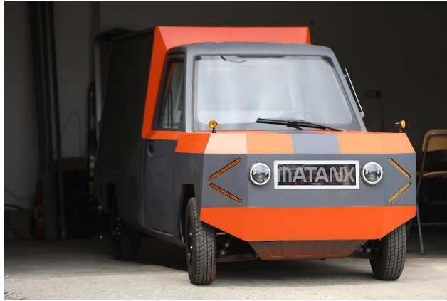
Figure 4: New electric vehicle MATANX with industrial hemp body [15]
