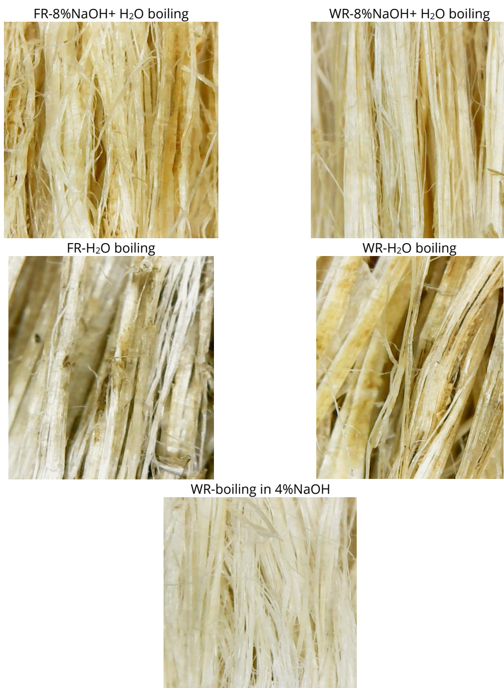
Figure 21: Dino-Lite microscopic images (magnification 50x) of longitudinal view of hemp fibre
