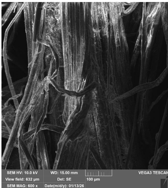
Figure 25. SEM micrographs of water retted hemp fibres boiled in 4% NaOH (specimen 5) under magnification of 200× and 1000×
