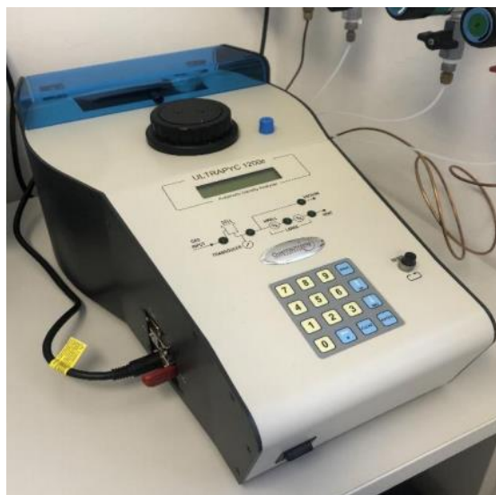
Figure 20: Automatic gas pycnometer for fibre density testing (Anton Paar)
