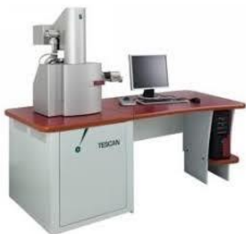
Figure 23: SEM Tescan Mira 3 LMU, Tescan and Sputter coater, Quorum
