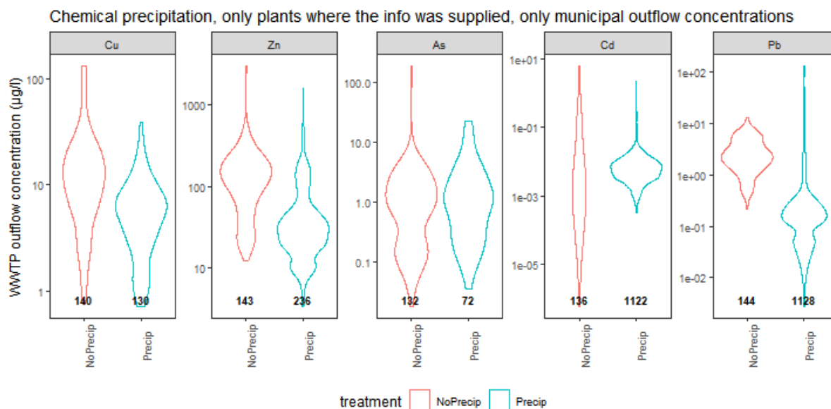
Figure 4: WWTP effluent concentrations by the presence / absence of a chemical precipitation step in the treatment technology. Number of measurements indicated.
