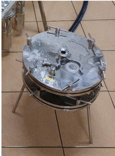
Figure 6. Filtration system developed and used by T. G. Masaryk Water Research Institute, Czech Republic.
