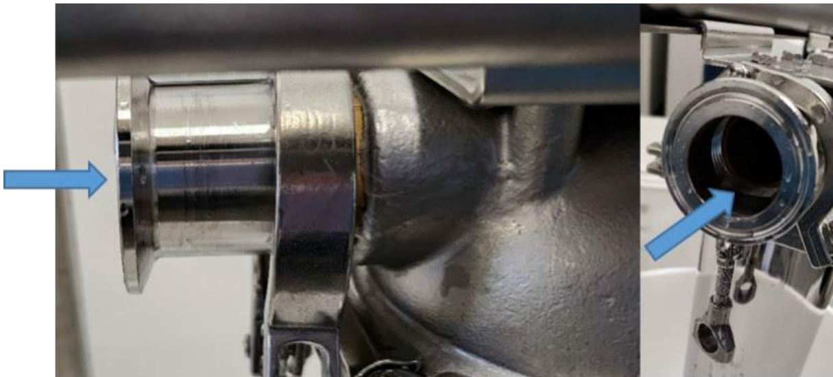
Figure 14. Inlet spout of the filter cartridge (photo: Environment Agency Austria).
